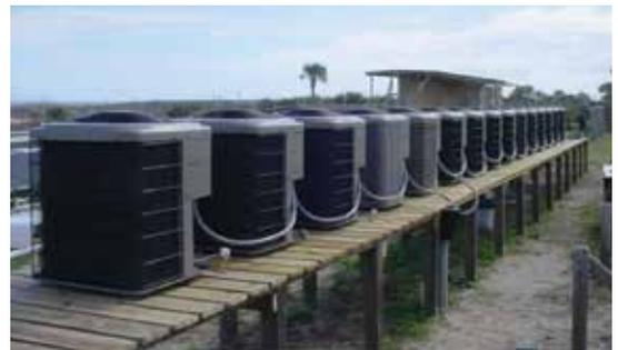
Reliability testing extends to extreme corrosive environments, both in labs and harsh field conditions, including coastal corrosion depicted above.
